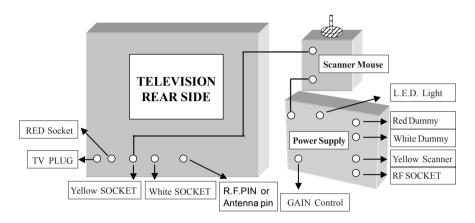
Please connect one of the two wires from the scanner to the audio video socket in the TV (Video socket color - yellow color) in the A.V mode in your TV.
