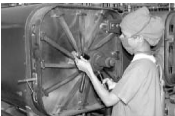
Fig : 4 - Unloading the autoclave
