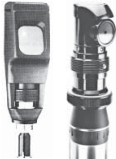
Fig. 6.1. Retinoscope heads, Two models
