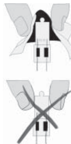
Fig 2.3. How and how not to handle bulbs
