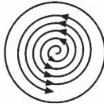
Fig 2.1. Shows the spiral path of the cleaning swab while cleaning circular optical elements
