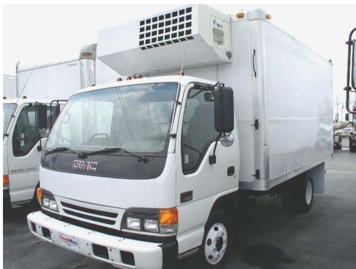
Figure 13. Collection Vehicle with Refrigeration Unit
