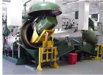
Tempico "Rotoclave" with automated cart tipper.
